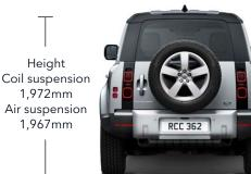
Rear wheel track Air suspension 1,702mm<sup>△</sup> Coil suspension 1,700mm<sup> $\Delta\Delta$ </sup>
